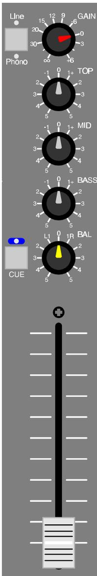
**Line / Phono** Inputselector. Normally is Line (CD, MD, tape), Pushed in is Phono (turntable). LEDs indicate which input is selected.
